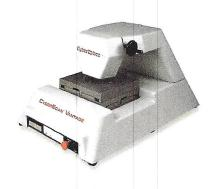
Vantage combines CyberOptics' latest laser technology with computer-driven x and y-axis stages to produce highresolution two- and three-dimensional profiles and scans. The system collects a series of height measurements to create a 2D profile, or performs a raster scan of the entire measurement site to produce a 3D topographical map.
